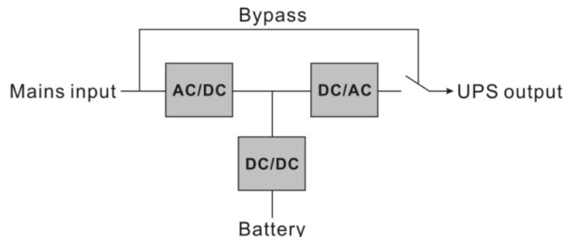
This product is a true online double-conversion UPS (Uninterruptible Power Supply). It provides perfect protection for critical load such as computer system. It can eliminate almost all mains power disturbances. The input AC current can be corrected to a wave following the mains voltage, so it is a high power factor system. Through the PWM control technology, the output voltage can be a pure & stable sine wave AC voltage.
