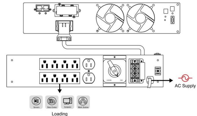
2) Change over the Maintenance Bypass Switch of PDU module from "INV." to "MAINT.," and disconnect the cable between PDU module and Main UPS. Main UPS can be sent to repair service. The load connected on PDU module will continuously be supplied by AC mains.
