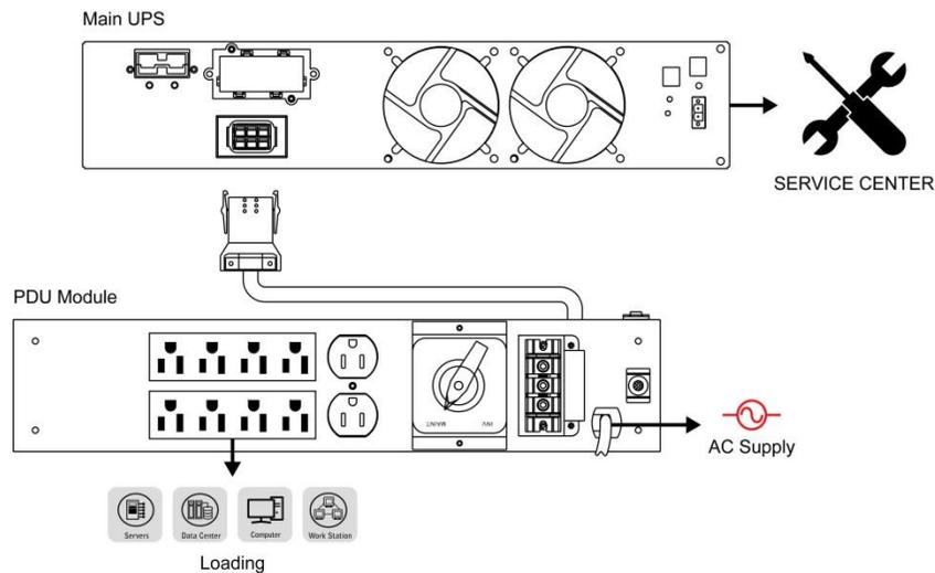
3) When UPS is returned from repair service, connect PDU module back to the main UPS. Change over the Maintenance Bypass Switch of PDU module from "MAINT." to "INV." and lastly press ON-button to turn on the UPS.
