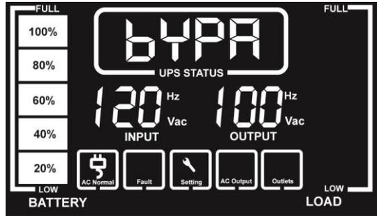
Step 2: The flickering figure would change to “120” after pressing the SELECT-button three times again.
